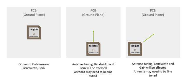
Figure 5: Examples of GNSS Ceramic Antenna Placement
