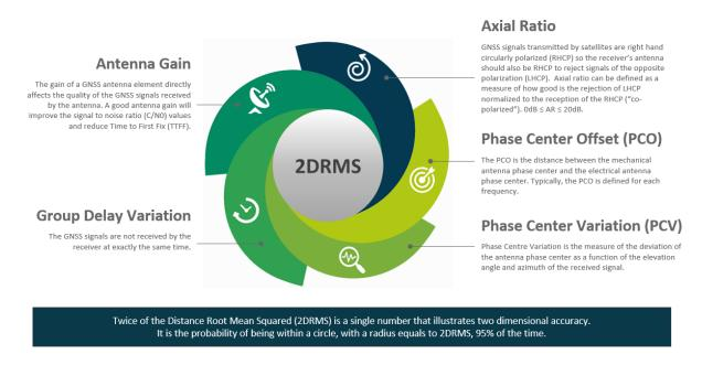
**Figure 3: GNSS Antenna Characteristics**
