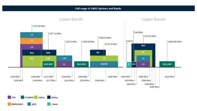
Figure 1: GNSS Constellation Types and Spectrum Bands
