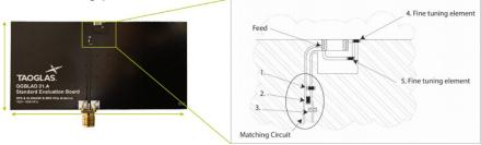
Figure 6: Example of internal chip antenna placement
